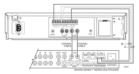
Figure 2. Connecting VCR to Multiplexer
